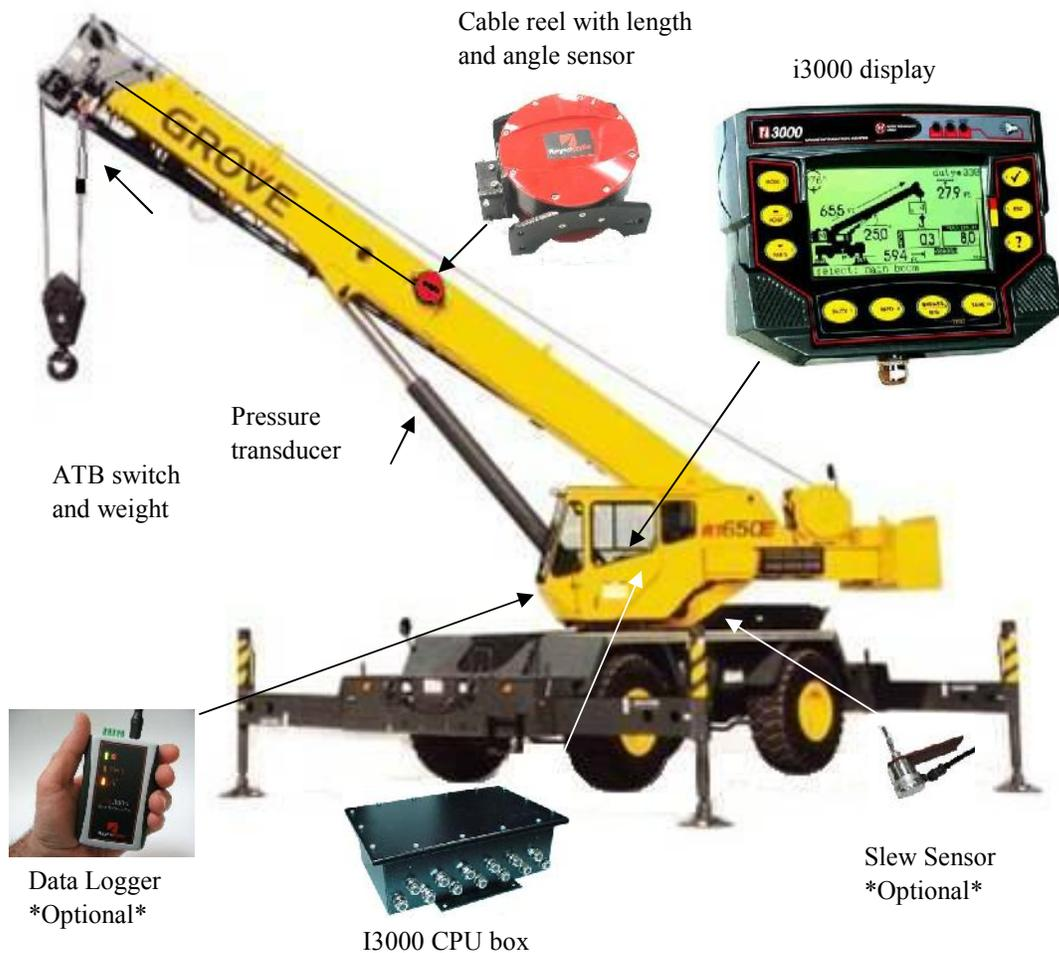
The i3000 pressure transducer system is a true Load Moment Indicator (LMI) because it actually measures the load on the boom from the pressure sensors mounted on the lift cylinder. This type of system is accurate, reliable, low maintenance, and easy to use. The i3000 has a powerful processor and large onboard memory that allows for large load charts and extra options such as data logging and range limiting.
