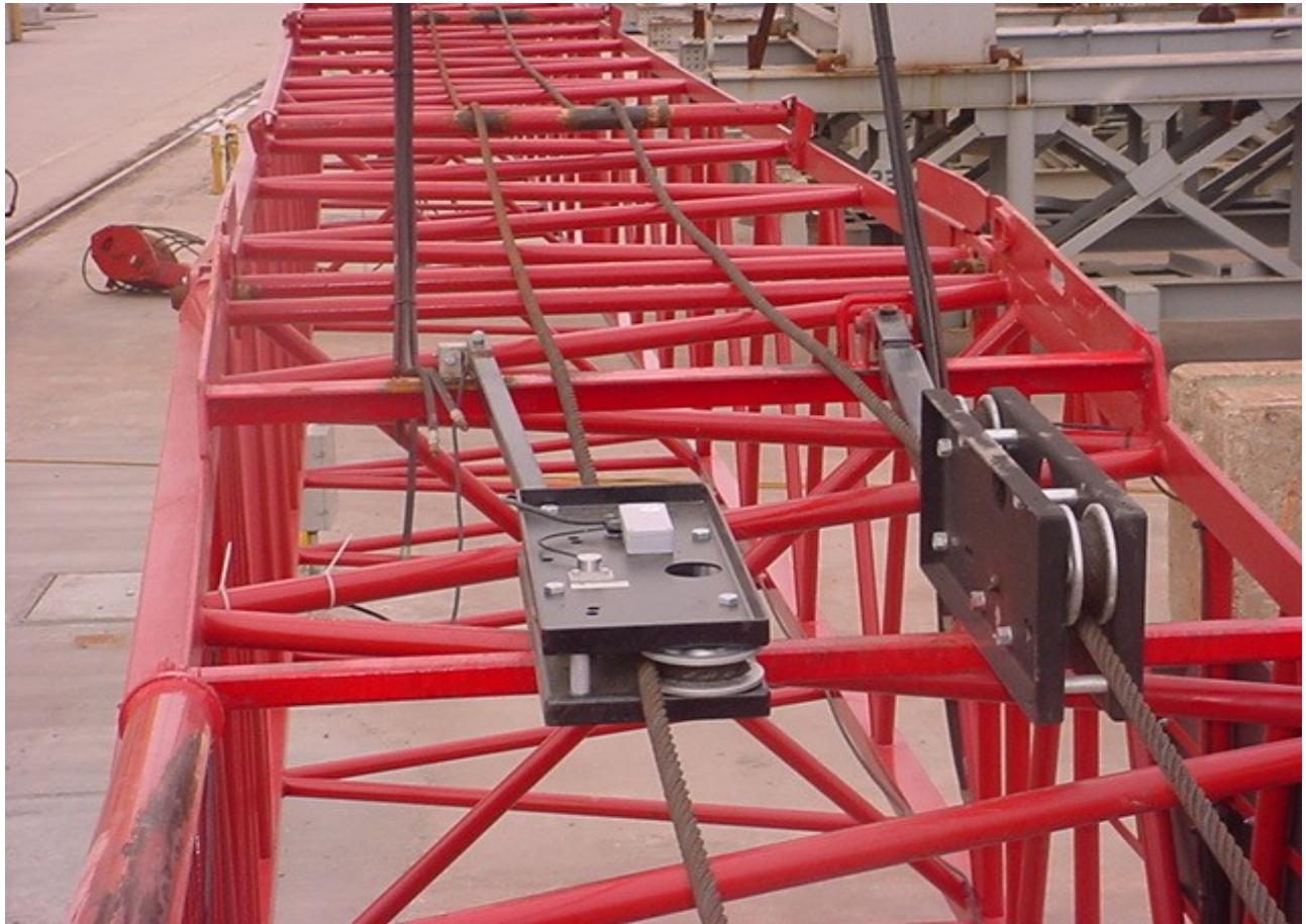
Dynamometers mounted side by side, vertical and horizontal on a lattice crane boom. Preferred method for lattice cranes with side by side winches.
