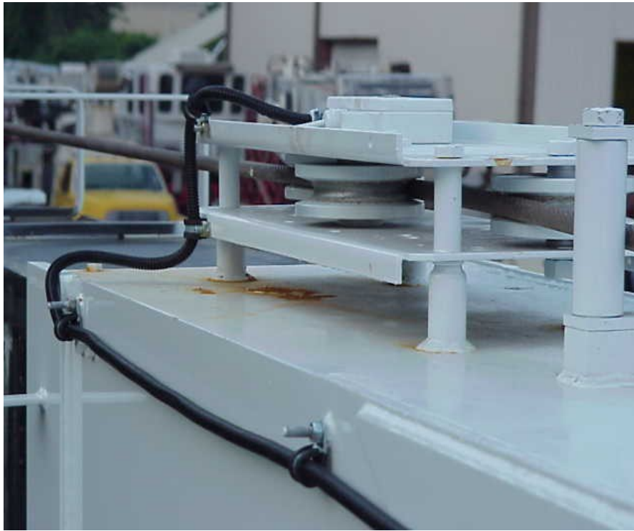
Dynamometer fix mounted on a telescopic hydraulic boom. Preferred mounting method for hydraulic cranes with boom mounted winch.
