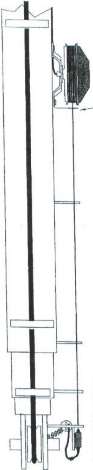
SWITCH AND JUNCTION BOX ARE FITTED ON A SPECIAL END GUIDE. PASS THE WIRE AS SEEN ON THE DRAWING.
