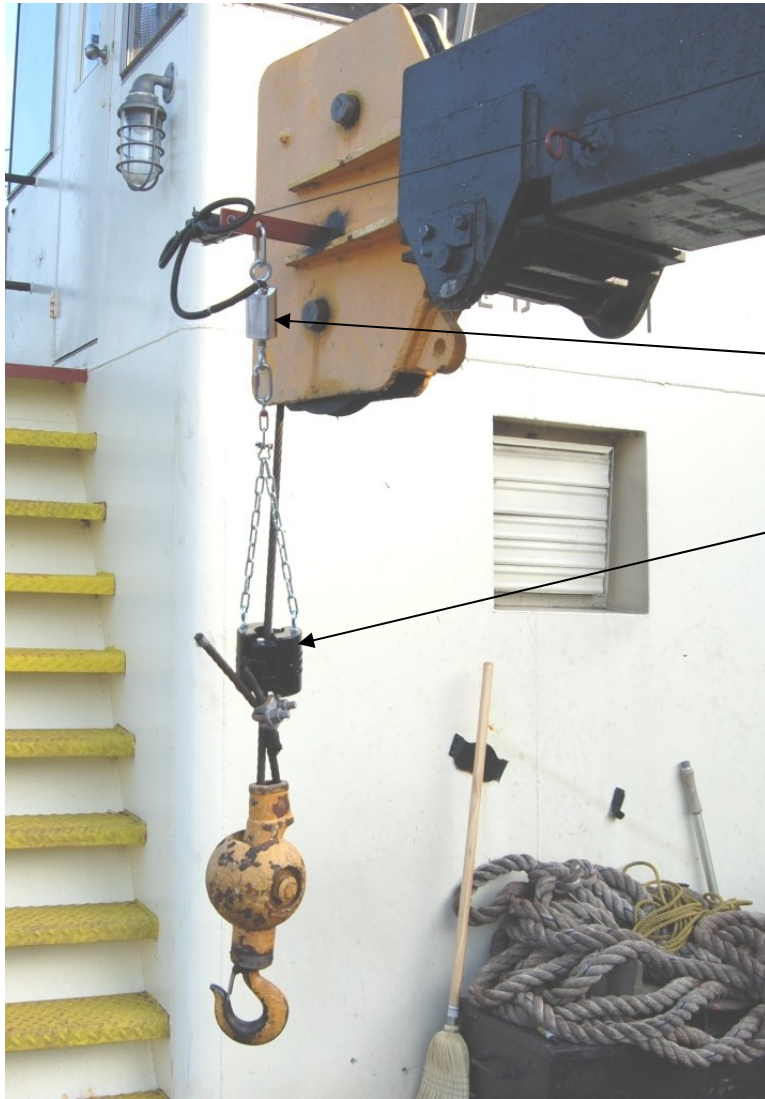
ATB Switch Mounted with weight and chain.
