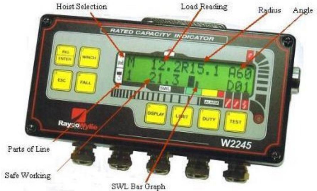
The W2245 LMI / RCI provides the operator with continuous display of the load, capacity, radius, and angle. The display shows a bar graph representing the percentage of safe working load. The system warns of approach of overload and anti-two-block. The internal relay is triggered for overload and ATB for use with a lock out system. The W2245 works on both lattice and hydraulic cranes.
