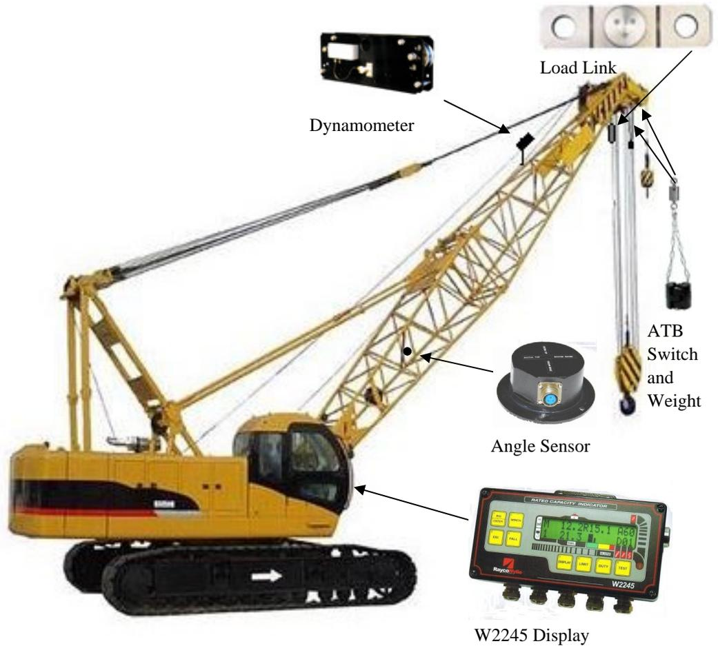
The W2245 used on lattice cranes can use a combination of one load link and a line rider (dynamometer) or two line riders. The W2245 works on lattice cranes with 360 degree load charts and provides the benefits of a rated capacity indicator at an affordable price. The system is easy to install and operate.
