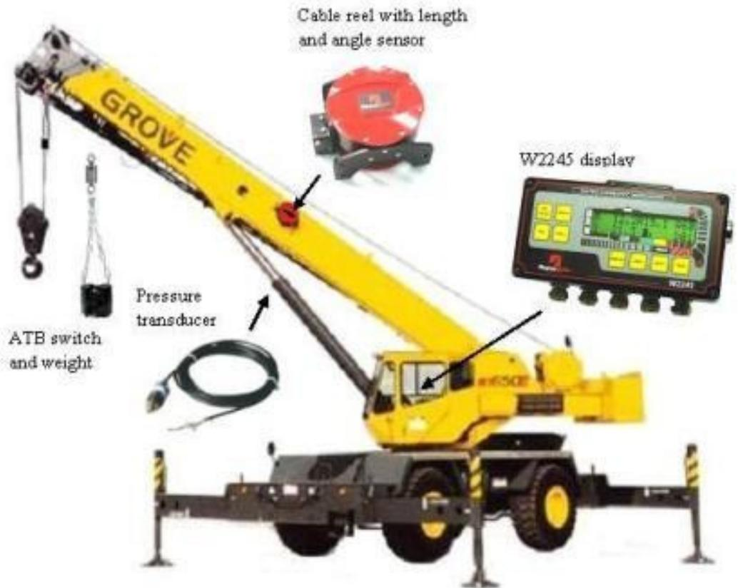
This is the most popular configuration for the W2245 system. For telescopic boom cranes with 360 degree load charts this is the most cost effective LMI system on the market. This is a true Load Moment Indicator (LMI) because it actually measures the load on the boom from the pressure sensors mounted on the lift cylinder. This style of system is accurate, reliable, low maintenance, and easy to use.
